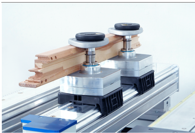
Mechanical clamps VCMC-S4-QUICK for clamping of frame parts
